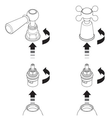
Before continuing please ensure that the water supplies have been isolated and drained where necessary. Always support the spout when removing/fitting cross handle/lever assemblies or ceramic cartridges.
