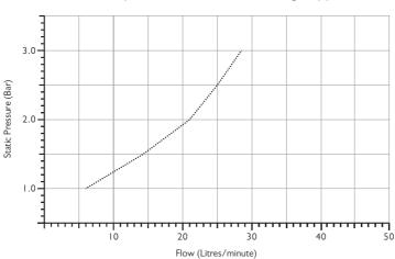
Note: Pressures shown are applied directly to the inlets; flow rates indicated are free flowing and may vary subject to restrictions created by installation, pipework, layout or application.
