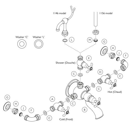
All joints should be 'hand tight only' until assembly and installation is finalised.
