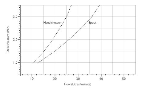
Note: Balanced pressures shown are applied directly to the hot and cold inlets; flow rates indicated are free flowing and may vary subject to restrictions created by installation, pipework, layout or application. Spout and hand shower tested separately.
