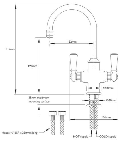
The recommended mounting surface opening is Ø30mm nominal.
