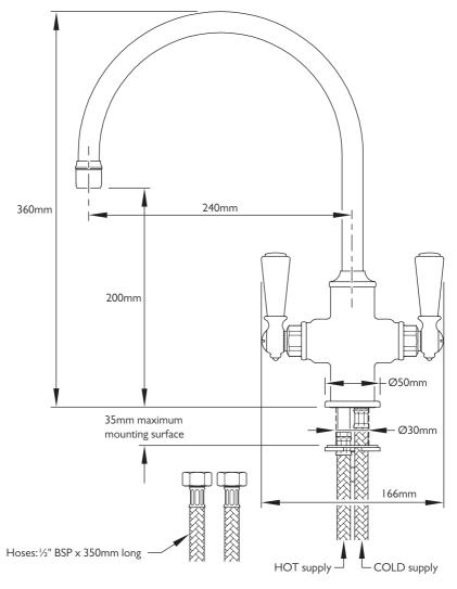
The recommended mounting surface opening is Ø30mm nominal.
