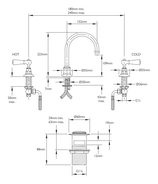
The recommended mounting surface opening for the spout is Ø32mm - Ø34mm. For flow valve mounting surface openings please refer to separate guide.
