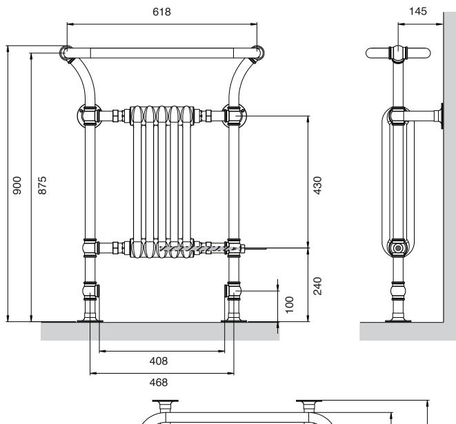
All dimensions are in mm and may vary + - 5mm as they are hand made, hand soldered and polished
