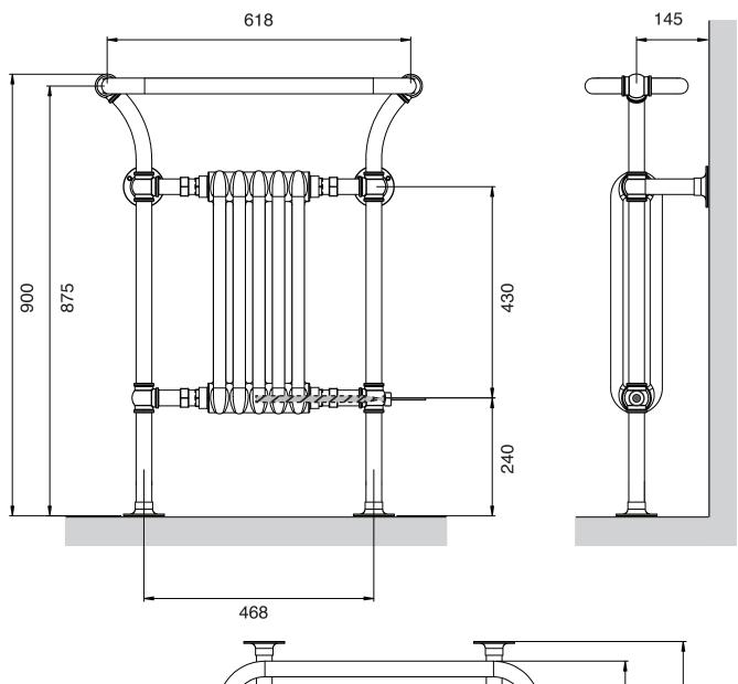
All dimensions are in mm and may vary + - 5mm as they are hand made, hand soldered and polished
