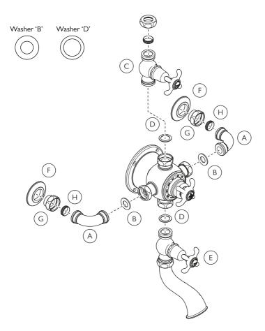
All joints should be 'hand tight only' until assembly and installation is finalised.
