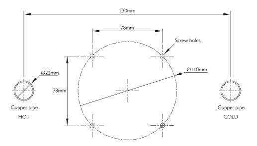
For dimensions of outlets for specific models please refer to the appropriate 'dimensions' section.
