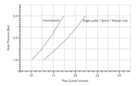
Note: Balanced pressures shown are applied directly to the hot and cold inlets; flow rates indicated are free flowing and may vary subject to restrictions created by installation, pipework, layout or application. The outlet temperature during testing was 38°C.
