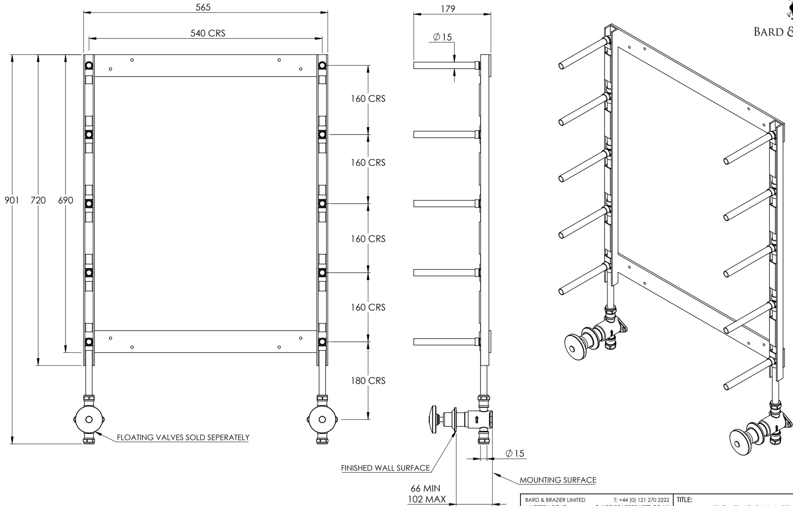
DO NOT SCALE DRAWING ALL DIMENSIONS ARE IN MILLIMETERS AND MAY VARY ± 5mm AS THEY ARE HANDMADE, HAND SOLDERED AND POLISHED
