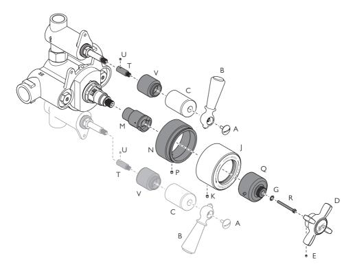
Lighter sections only relevant on 8736 models. Extension kit components are shaded
