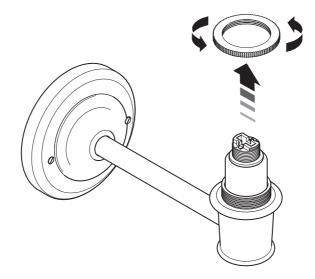
6 Locate and screw the stem of the lamp in place.
