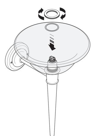
10 Gently push the bulb in place before screwing the protective shroud onto the housing.
