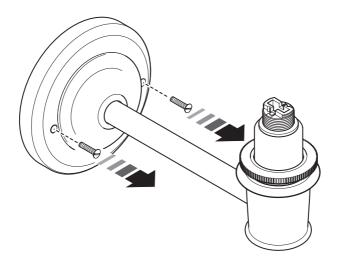
2 With the raised screw holes facing you, place the mounting plate against a suitable mounting surface. Using a spirit level, ensure that the raised screw holes are horizontal. Mark the location of the two slotted holes on the mounting surface. Drill two suitable holes for the required fixings. Wall plugs and screws are supplied with the lamp. Feed the supply cable through the central hole in the mounting plate. Secure the mounting plate using suitable fixings.
