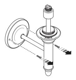
2 With the raised screw holes facing you, place the mounting plate against a suitable mounting surface. Using a spirit level, ensure that the raised screw holes are horizontal. Mark the location of the two slotted holes on the mounting surface. Drill two suitable holes for the required fixings. Wall plugs and screws are supplied with the lamp. Feed the supply cable through the central hole in the mounting plate. Secure the mounting plate using suitable fixings.
