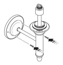
5 Unscrew and remove the circular shade retainer from the lamp.
