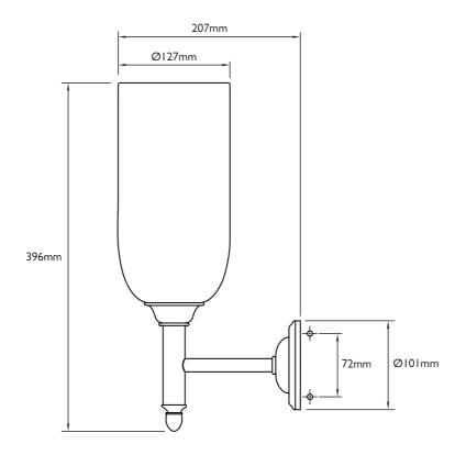
I Unscrew and remove the two screws from the front of the lamp. This will release the mounting plate at the rear.
