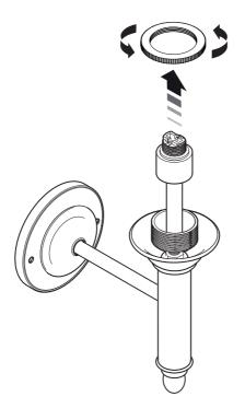
6 Locate the shade onto the lamp body.
