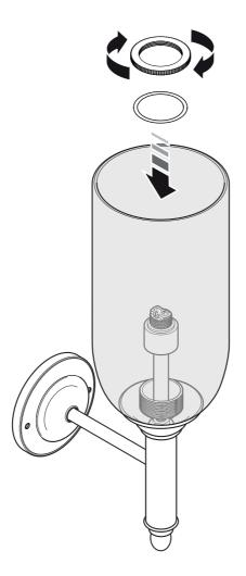
9 Gently push the bulb in place before screwing the protective shroud onto the housing.
