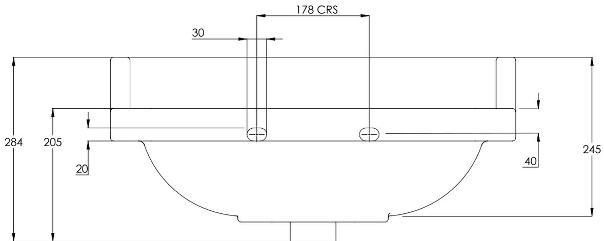
ALL SHOWN DIMENSIONS ARE IN MILLIMETERS AND ARE SUBJECT TO STANDARD CERAMIC TOLERANCES.
