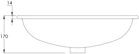
ALL SHOWN DIMENSIONS ARE IN MILLIMETERS AND ARE SUBJECT TO STANDARD CERAMIC TOLERANCES.
