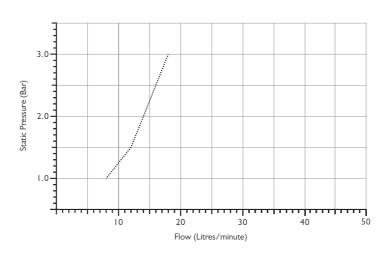
Note: Balance pressures shown are applied directly to the hot and cold inlets; flow rates indicated are free flowing and may vary subject to restrictions created by installation, pipework, layout or application.
