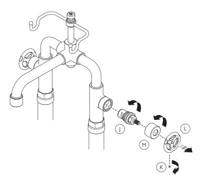
Before continuing please ensure that the water supplies have been isolated and drained where necessary.
