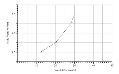
Note: Balance pressures shown are applied directly to the hot and cold inlets; flow rates indicated are free flowing and may vary subject to restrictions created by installation, pipework, layout or application.
