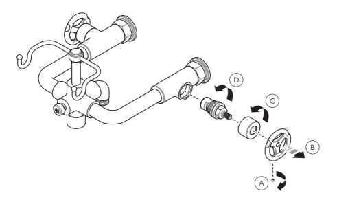
Before continuing please ensure that the water supplies have been isolated and drained where necessary.
