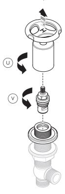
Before continuing please ensure that the water supplies have been isolated and drained where necessary.
