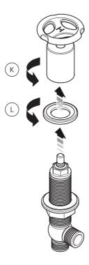
Before continuing please be aware that on lever models it is important to keep the flow valve bodies and lever assemblies together as supplied. Do not swap the lever assemblies from hot and cold valves.
