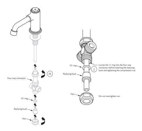
9 Locate the four way connector and tighten the upper locking nut (H). Ensure that the 'o' ring is located into the four way connector (J) before inserting the reducing bush. Tighten the compression nut.
