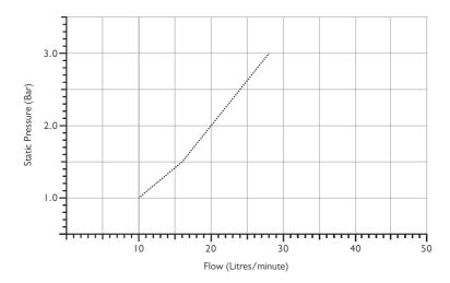
Note: Balance pressures shown are applied directly to the hot and cold inlets; flow rates indicated are free flowing and may vary subject to restrictions created by installation, pipework, layout or application.
