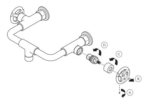
Before continuing please ensure that the water supplies have been isolated and drained where necessary.
