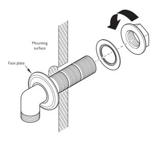
Note: Before fitting the wall outlet ensure that a rubber 'o' ring is fitted to the rear of the face plate. This is factory fitted, though may have worked loose during transit.
