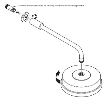
I To aid installation the shower rose and arm can be disassembled as shown above. Ensure that the set screw is removed completely to avoid damage to the 'o' rings. The set screw can be removed using a 2.5mm hexagonal key.
