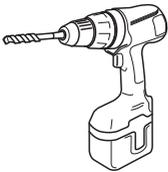
Powered drill with  $\varnothing$ 6mm drill bit
