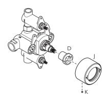
5 Remove the thermostatic cartridge cover (J) by unscrewing set screw (K) using a 1.5mm hexagonal key. Temperature stop (D) can be pulled off.
