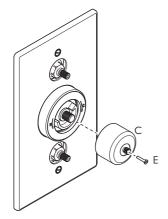
3 Remove the override (C) by unscrewing and removing screw (E).
