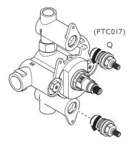
2 After installing the replacement flow cartridge, unscrew the centre screws in the non-return valves and assemble the valve in reverse order.
