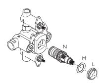
7 To remove the thermostatic cartridge, unscrew and remove locking nut (L). Remove anti–rotation washer (M) and pull out cartridge (N). To help with cartridge removal, it is recommended you fit override (C) with screw (E) to make pulling the cartridge out easier.
