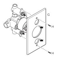
4 To remove the facing plate (G) unscrew and remove fully the 2 fixing screws (H). Carefully prise the facing plate off the wall using a flat bladed screw driver (the gasket is reusable).
