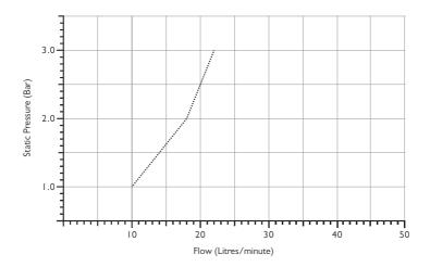
Note: Balance pressures shown are applied directly to the hot and cold inlets; flow rates indicated are free flowing and may vary subject to restrictions created by installation, pipework, layout or application. The outlet temperature during testing was 38°C.
