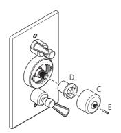
Remove the override (C) and temperature stop (D) by unscrewing and removing screw (E).
