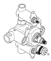
I Isolate the hot and cold water supplies before the shower valve. With the facing plate, lever assemblies, cartridge cover and temperature stop removed, you can see the non-return valve housing(s). Using a 17mm spanner or socket, unscrew and remove the non-return valve housing(s) (R).
