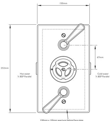
230mm x 120mm aperture behind face plate for maintenance access
