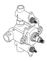
With the water supplies isolated by the non-return valves, using a 17mm spanner or socket, unscrew the flow cartridge(s)
