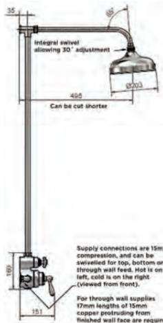
Supply connections are 15mm compression, and can be swivelled for top, bottom or through wall feed. Hot is on left, cold is on the right (viewed from front).
