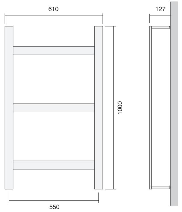
Test pressure: 6 BAR Max working pressure: **3 BAR** Max working temperature: 100°C Connections: 1/2" FI Heat output determined in accordance with EN 442 Btu/hr @ Delta 60: 2839 1000 Height over flange: Width over flange: 610 Overall projection: 127 Pipe centres: 550 Tube mm:
