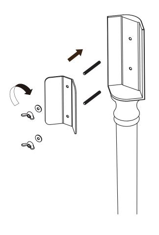
Prepare both legs by locating and screwing the threaded bars into each of the holes on the back of the console legs.
