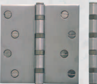
Slimline projection X1227 H x W x D (mm): 102 x 102 x 2.5 H x W x D (in): 4 x 4 x 3/32 Butt Dia. 10mm Max loading 120kg Based on 3 hinges per door
