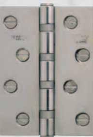
Slimline X1226 H x W x D (mm): 102 x 76 x 2.5 H x W x D (in): 4 x 3 x 3/32 Butt Dia. 10mm Max loading 120kg Based on 3 hinges per door
