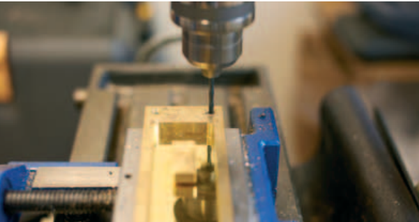
Drilling flush plates
