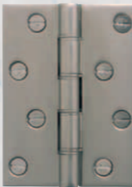
Traditional DPBW Butt X1230 H x W x D (mm): 102 x 76 x 3.5 H x W x D (in): 4 x 3 x 1/8 Butt Dia. 10mm Max loading 40kg Based on 3 hinges per door
