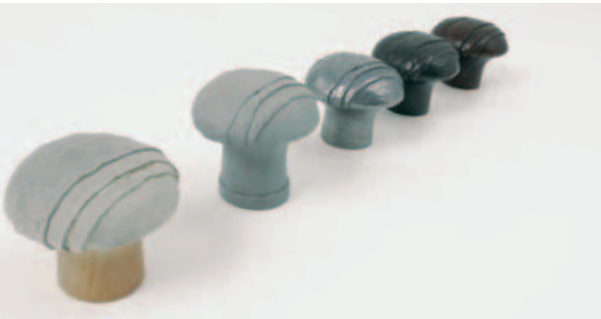
Lead and timber master, to PU interim master, to finished product
